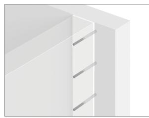
Fig. 11: Schöck Dorn: Connection wall-wall (face-flank)
