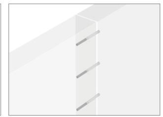
Fig. 12: Schöck Dorn: Connection wall-wall (face-face)
